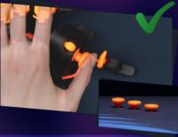
Change the angles between **OMRON SWITCH KEY** towers-slightly loosen the screws of key towers until each tower fits your fingers naturally. Remember - adjust the keypad to your hand and not vice versal **TOWERS COMPLEMENT YOUR NATURAL CLAW GRIP OF YOUR FINGERS.** Even if you have loooong fingers you will find your best fit.
