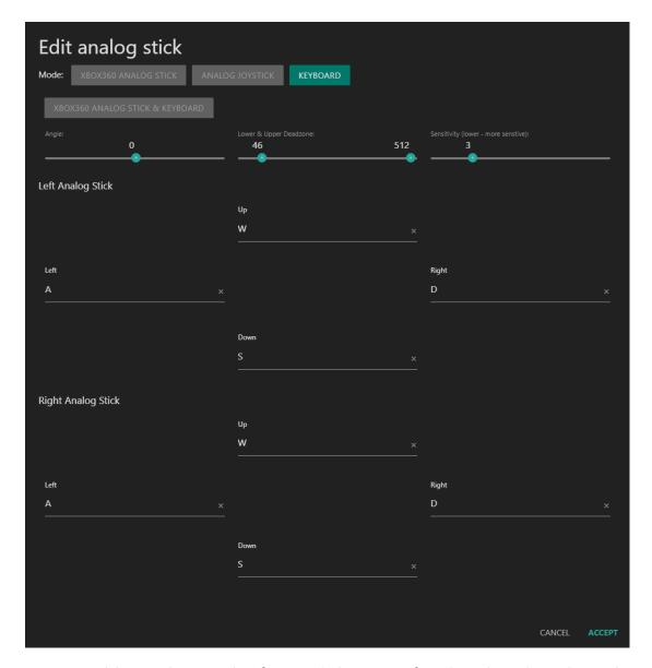
It is possible to change the forward direction for thumbstick with **angle slider** up to 180° in each direction.
