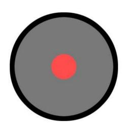
Lower deadzone is an area in the center of the thumbstick that won't recognize input if the stick is moved within it. The higher the value, the bigger the circle is in the center where thumbstick movement won't register.
