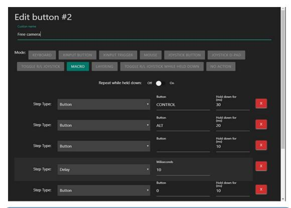
Macro function is available only in software profiles! Currently it is not possible to save Macro in on-board memory due to the Teensy PCB limitations.
