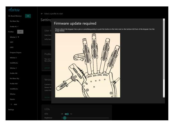
Now take the included hex screwdriver and press the reset button (see the picture). The keypad will restart.
