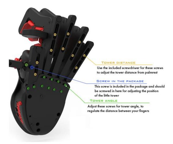
By using the included Hex screwdriver, it is possible to adjust each key tower position for your hand.
