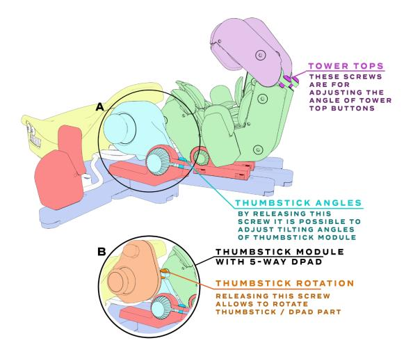
By using the included Hex screwdriver, it is possible to adjust key and thumb module positions for your hand.
