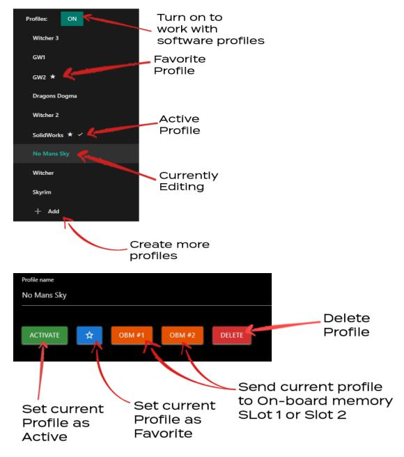
Any software profile can also be sent to On-board memory, by pressing **OBM#1** or **OBM#2**. Note that Macro will not work in on-board memory profiles.
