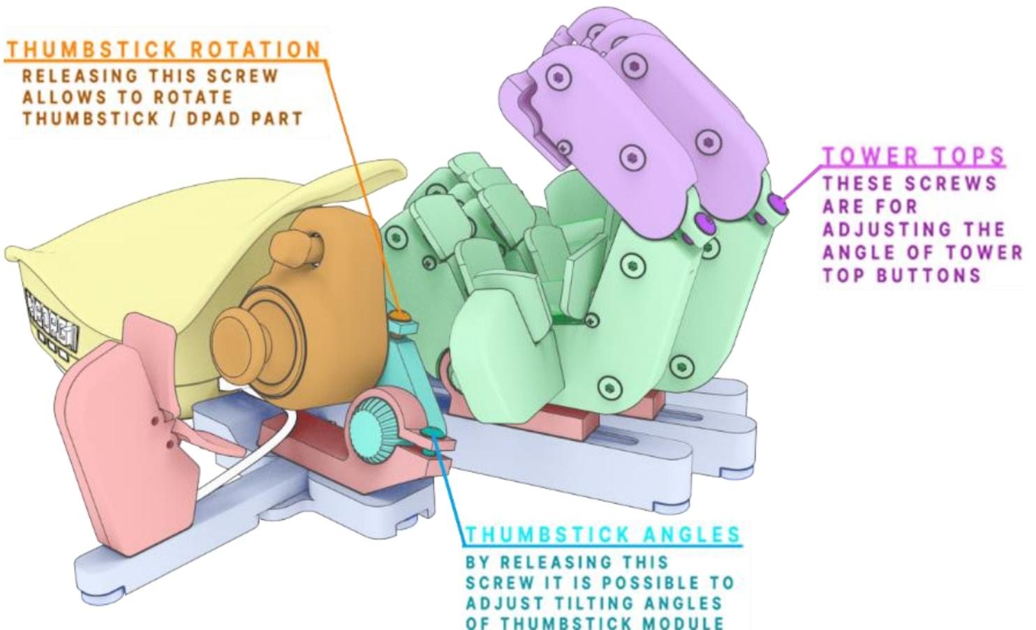
By using the included Hex screwdriver, it is possible to adjust key and thumb module positions for your hand.
