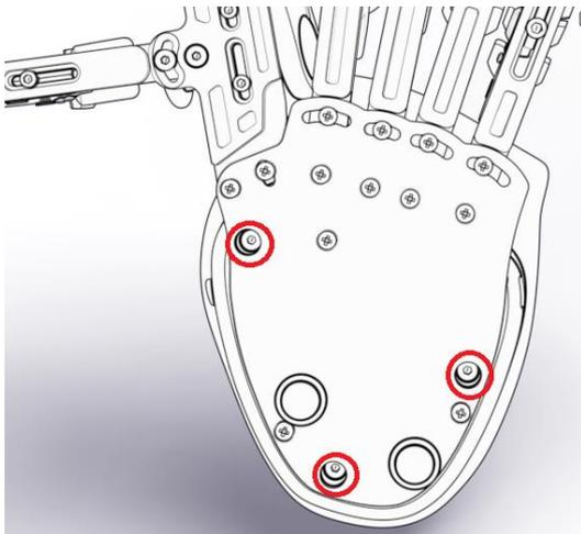
To fix the wire issue, open the palmrest by unscrewing the 3 deep recessed screws underneath the Azeron, then lift the palmrest off your keypad.
